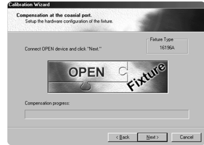
Figure 12. Calibration wizard (open compensation)
